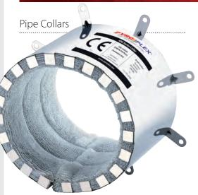
Pyroplex® CE Marked Pipe Collars reinstate the fire resistance of walls and floors that have been penetrated by flammable pipes. The Pyroplex full range of CE Marked Collars – 2 hour and 4 hour, are available for use on plastic pipes from 25 to 400mm.
