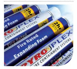
Pyroplex® Fire Rated Expanding Foam is suitable for sealing gaps around doors and window frames, using secondary fire sealing media around services, such as metallic cable trays and general service penetrations. Pyroplex Fire Rated Expanding Foam has a European Classification of El120 in accordance with BS EN 13501-2: 2007.
